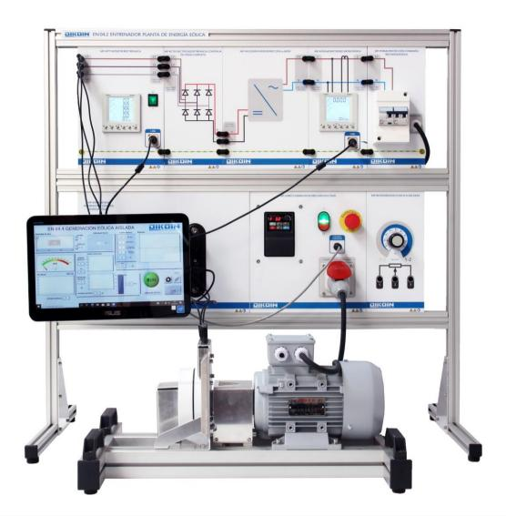
With this equipment, we emulated the behavior of a wind turbine in a practical and didactic way. An electric motor acts as the blades and bush of a wind turbine, dragging a three-phase synchronous generator of permanent magnets, which transforms the mechanical energy transmitted to the shaft into electrical energy at the output.
